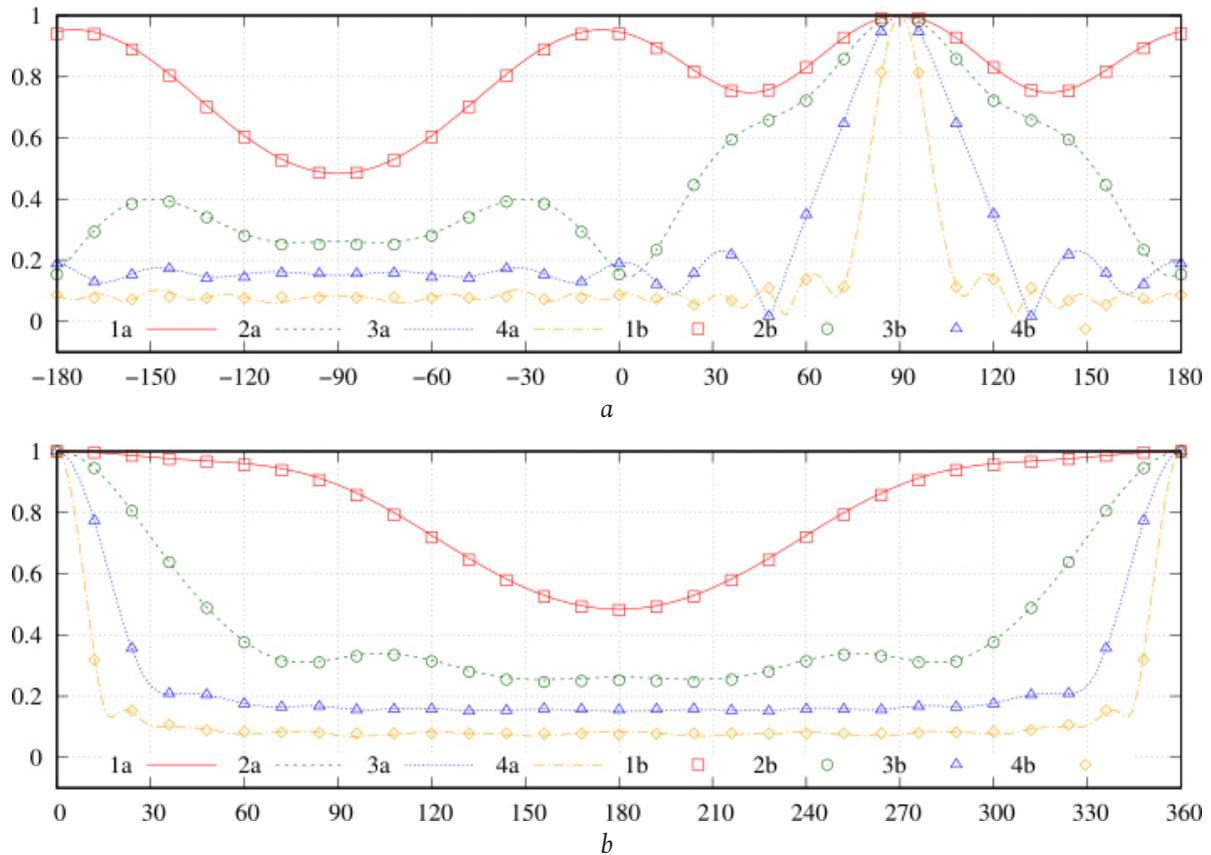
Fig. 3. Comparison of normalized DR in the meridian and azimuth planes:  $a$  - TP method;  $b$  - FEM; RWG method; 1 -  $r = 0,25\lambda$ ; 2 -  $r = 0,5\lambda$ ; 3 -  $r = 1\lambda$ ; 4 -  $r = 2\lambda$
