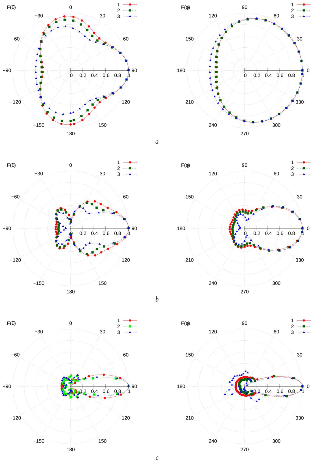
Fig. 4. Normalized meridian (left) and azimuthal (right) RPs for structures 1–3 (curve number corresponds to structure number):
